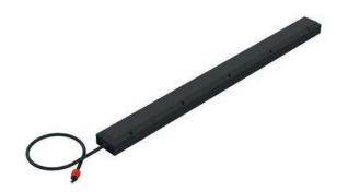
The 270 SERIES side-scan is a robust fully moulded construction, with a very wide bandwidth. With a narrow beam in the alongtrack axis and wide beam in the across-track axis suitable for most sea-floor mapping and other high directivity applications. A deepwater version, capable of operating down to 2000 metres, is available to special order. • FREQUENCY 65 KHZ
