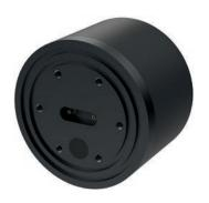
Designed for use in transponder beacons, data communication, acoustic release mechanisms and long-range base line systems, the T413 is a versatile transducer combining broadband transmission and reception over a hemispherical beam pattern. The overmoulded design onto an anodised aluminium
