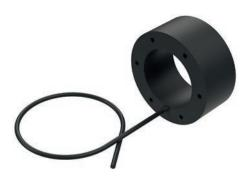
The T170 is one of a range of Free Flooded Ring transducer. Utilising the latest ceramic technology, the FFR concept is ideally suited for high power, broadband, low frequency sound generation. Another advantage of the design is its ability to operate down to full ocean depth at maximum efficiency.
