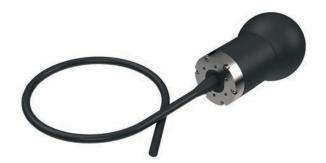
The D/17/BB is a highly efficient omnidirectional transducer with a 3dB bandwidth from 12 kHz to 27 kHz. The D/17/BB transducer is ideally suited for use in broadband noise systems, long-range transponder and voice/ data communications.
