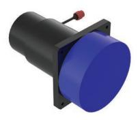
The T296 is a single tonpilz transducer offering a high power, broad band performance. With a nominal operating frequency range from 1 kHz to 6 kHz, these transducers can be configured to form half lambda spaced arrays. The robust design is tolerant of both dynamic and static
