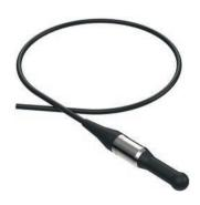
The D/140/H is a true spherical and balanced element combined with a low noise differential pre-amplifier. Signals can be transmitted along cable lengths up to 250m, without any degradation. The pre-amplifier gain options of 20, 30 and 40 dB (pre-set during manufacture) are to suit customer requirements.
