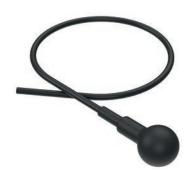
The D/45 spherical transducer is a versatile design providing omni-directional transmit and receive characteristics over a wide frequency range. The fully moulded construction, coupled with the inherent strength of the PZT ceramic sphere, achieves a robust, lightweight and corrosion free design making it the ideal choice as a high-power projector.
