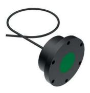
The Type T38 is a precision echo sounder transducer designed for use in hydrographic or scientific applications where an accurately defined, narrow beam pattern is required. Operating at 120 kHz the multi-element array is configured to achieve two, highly directional, conical beam patterns with low side lobe levels. The transducer enables the beams to
